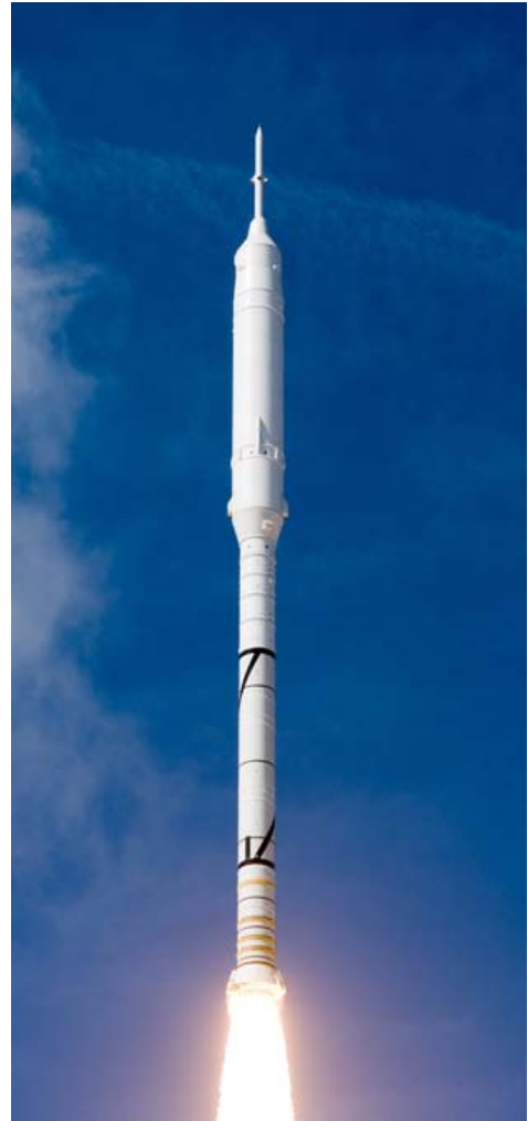
Figure 1. The Ares I-X Flight Test Vehicle (FTV) was successfully launched from Launch Complex 39B at 11:30 a.m. EDT on October 28, 2009. The 327-foot-tall vehicle produced 2.96 million pounds of thrust at liftoff. (NASA)
