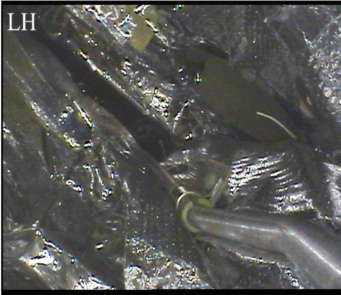
Figure 11-4 Boroscope view of LH Xo 378 purge vent after repositioning of blanket (SPC # 90790)
